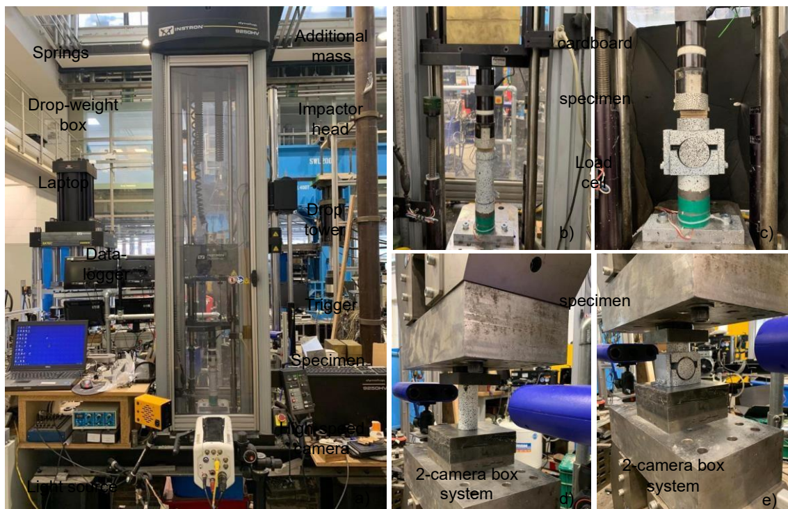
Figure 3. Impact tests: a) Impact loading rig, b) Impact compressive tests, c) Impact splitting tensile tests, d) quasi-static compressive tests, e) quasi-static splitting tensile tests.
