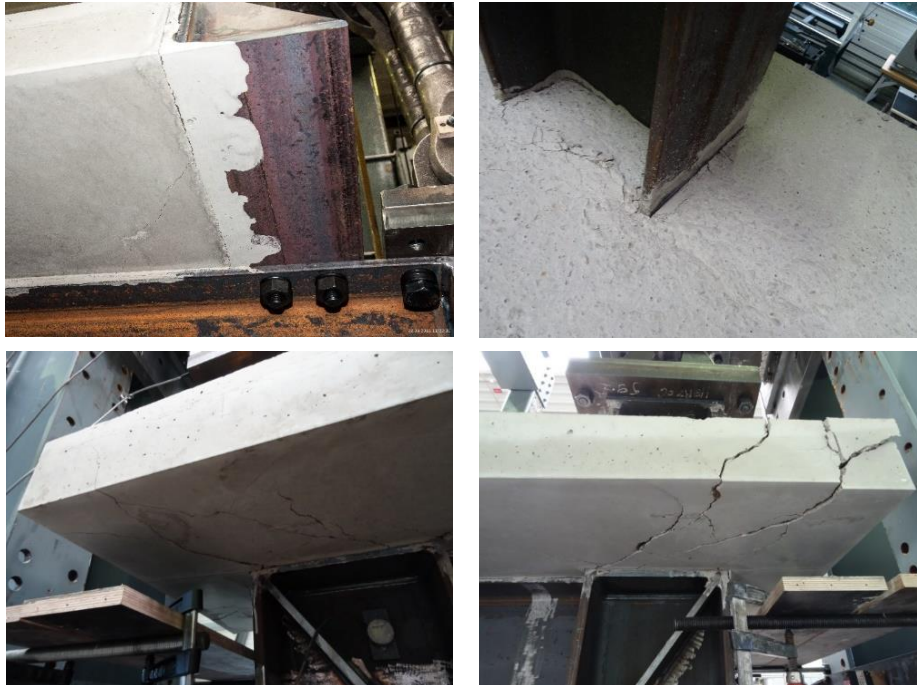
Figure 6. Damage evolution of steel-concrete specimens.
