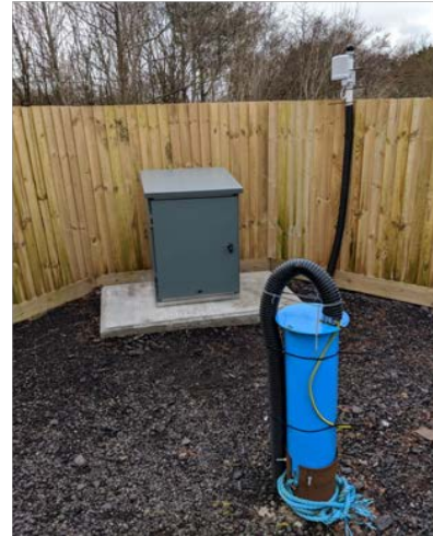
Figure 3: Photographs of two UDDGP microseismic stations. A) a broad-band seismometer station powered by 12V deep-cycle batteries, with continuous recharging via solar-panels. B) a borehole geophone station using mains power and backup batteries. The wellhead standpipe is blue and the black conduit carries the geophone cable underground into the instrumentation cabinet.
