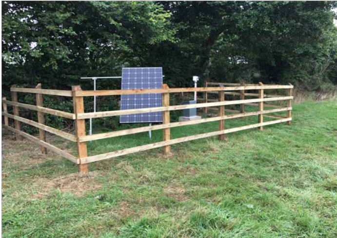
Figure 3: Photographs of two UDDGP microseismic stations. A) a broad-band seismometer station powered by 12V deep-cycle batteries, with continuous recharging via solar-panels. B) a borehole geophone station using mains power and backup batteries. The wellhead standpipe is blue and the black conduit carries the geophone cable underground into the instrumentation cabinet.
