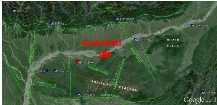
Figure 2. Major tectonic features of the region around the city of Guwahati. Locations of the fault lines taken from Baruah and Hazarika (Baruah and Hazarika 2008).
