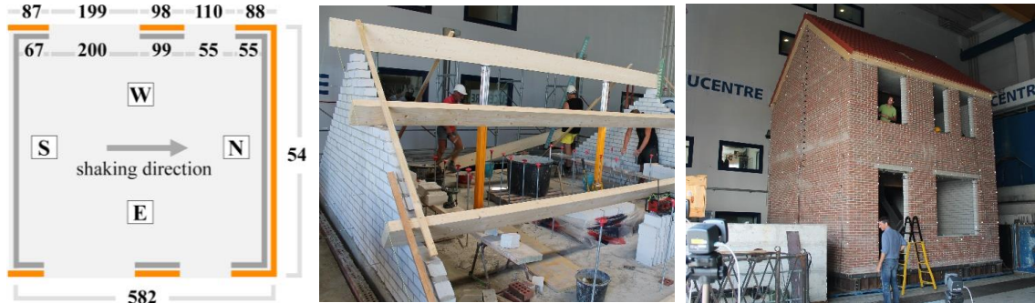
Figure 6. Plan (in cm) and experimental configuration of EUC-BUILD1 (Graziotti et al. 2017)
