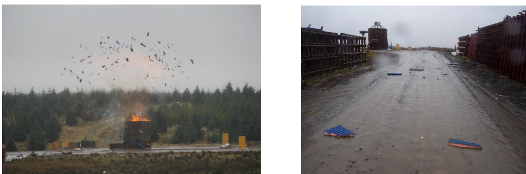
Figure 12 – Response of frangible panels
