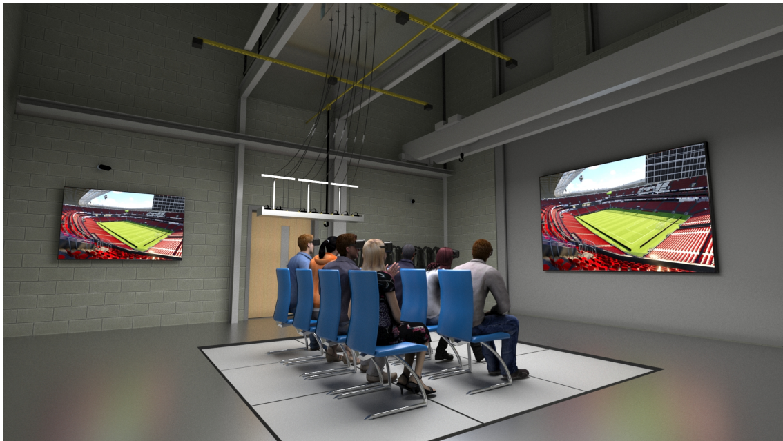
Figure 2: VSimulator in 'stadium mode' using virtual reality and controlled motion of the 4mx4m instrumented platform.
