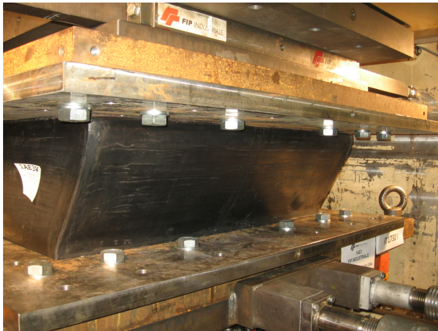
Figure 13. LRB prototype under testing.
