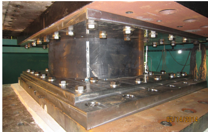
Figure 2. The HDRB prototype under compression stiffness test.
