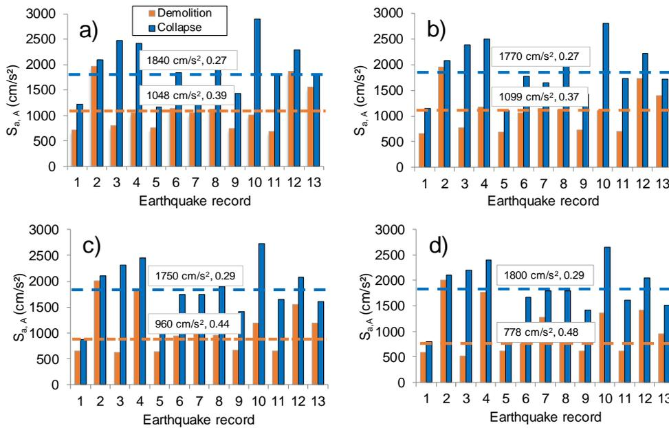
Figure 12. Comparison of  $S_{a,A}$  and  $S_{a,D}$  corresponding to different  $RIDR_o$  for model M2: a) 0.1%; b) 0.5%, c) 1.0%, d) 1.4%.
