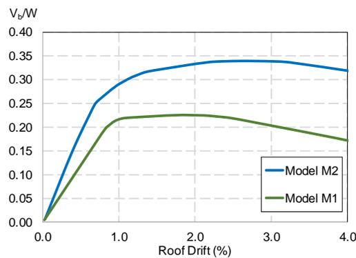
Figure 2. Comparison of capacity curves for building models M1 and M2.
