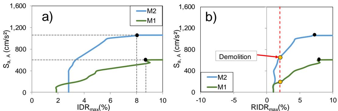
Figure 5. Comparison of post-mainshock IDA curves corresponding to models M1 and M2 under the aftershock recorded at Sylmar station: a)  $IDR_{max}$ , and b)  $RIDR_{max}$ .
