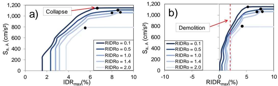
Figure 4. Post-mainshock IDA curves to obtain the aftershock collapse capacity of the M2 building model under the aftershock recorded at Sylmar station: a)  $IDR_{max}$ , and b)  $RIDR_{max}$ .
