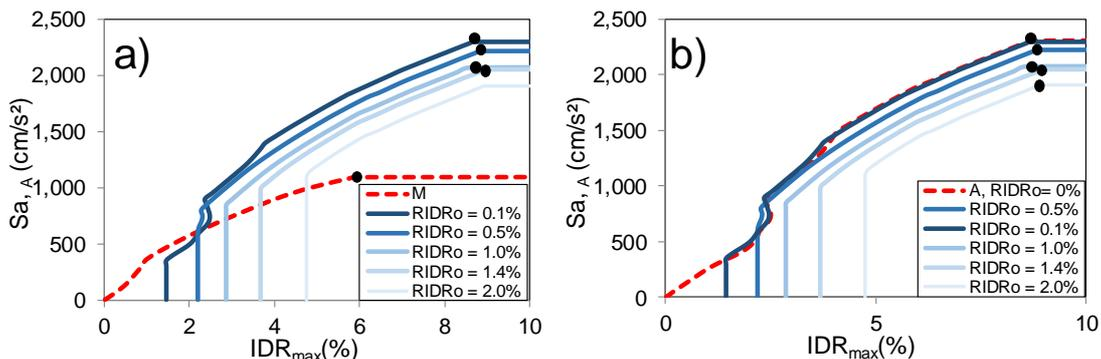
Figure 7. a) comparison of mainshock IDA and post-mainshock IDA curves; b) comparison of post-mainshock IDA curves with  $RIDR_o=0$  and post-mainshock.
