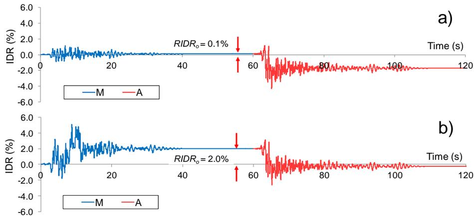
Figure 8. Re-centring behaviour observed in third-story drift time-history for two levels of  $RIDR_o$ : a) 0.1%, and b) 2.0%.
