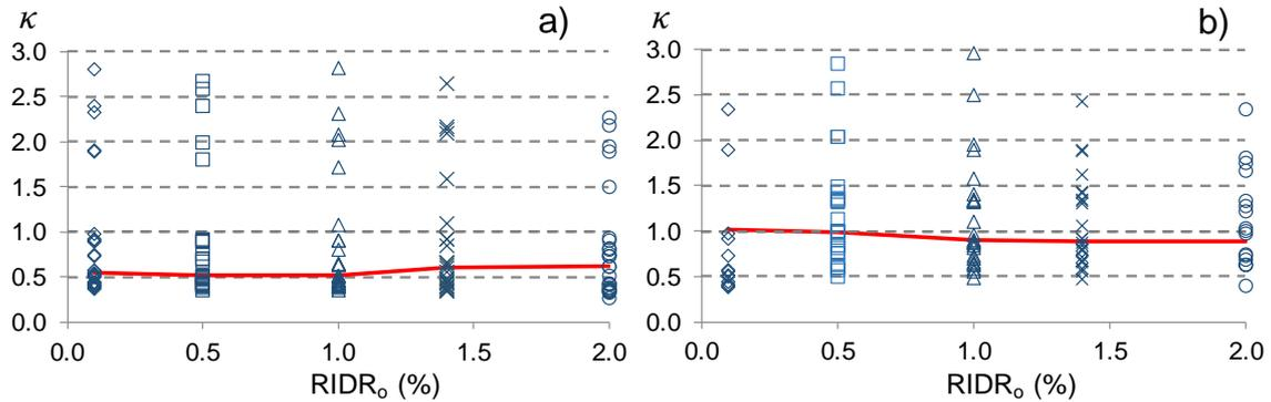
Figure 10. Residual capacity index computed from the mainshock-aftershock pairs for both models considered in this study: a) model M1; b) model M2.
