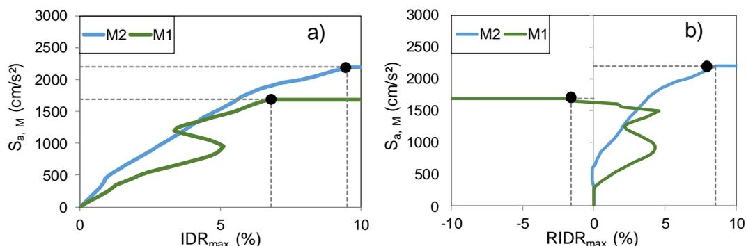
Figure 3. IDA curves to obtain the mainshock collapse capacity of the models M1 and M2 under Sylmar (comp. 288) record: a)  $IDR_{max}$ , and b)  $RIDR_{max}$ .
