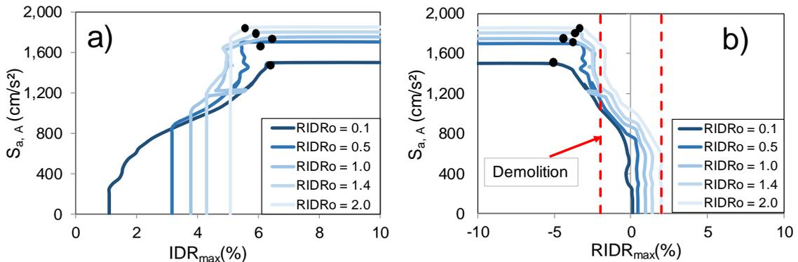
Figure 9. Post-mainshock IDA curves to obtain the aftershock collapse capacity of model M2 under the aftershock recorded at Sylmar station: a)  $IDR_{max}$ , and b)  $RIDR_{max}$ .
