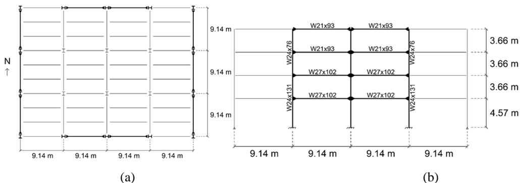
Figure 1. Case-study steel framed-building considered in this study: a) Plan view, b) East-West elevation.
