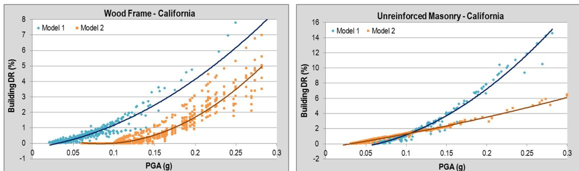
**Figure 1.** Anonymised examples of the different vulnerability curves assigned by independent models for two common building types in California.
